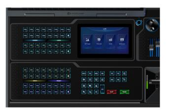
User-programmable LCD function buttons satisfy all your operation requirements in the field. Function names, pages and more can be clearly shown on the buttons, and the button skins and styles can be customized as you wish.
