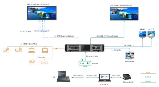
Figure 4-4 PGM only mode (P10+U5+PixelFlow)
