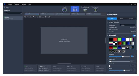
Step 3 If the device model is the Q8, click + to add screens; if the device model is the P20 and P10, the number of screens is fixed and you can skip this step.
