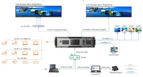
Figure 4-2 PGM only mode (P20+U5+PixelFlow)
