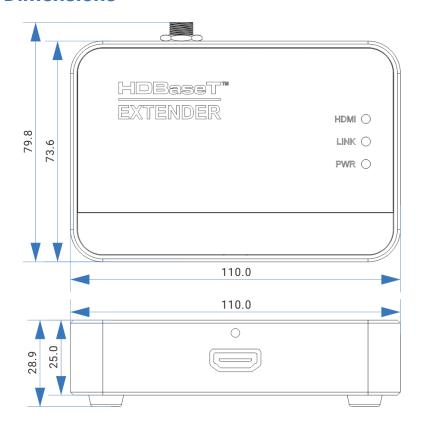
Tolerance: ±0.3 Unit: mm
