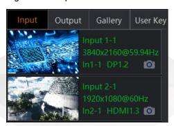
Step 3 Click in an input area, and the system will capture the current frame of the selected input source automatically. The captured image can be saved in Triton, as shown in Figure 7-47.
