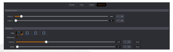
Step 5 Select the blending edge and enable the feathering as required.
