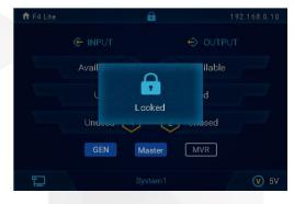
When the device front panel is locked, button presses will have no effect.
